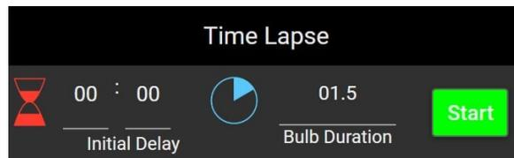
When the camera is in bulb mode, the timer tab can also be used to perform bulb shots with a specified duration. The Start button in the Bulb section will only take a single shot. However, time-lapse can be combined with bulb mode to perform a time-lapse with each bulb duration set by the shot duration.
