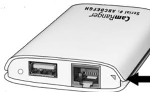
The bottom cover is the side with the CamRanger serial number. Simply grasp the side edge/corner of the cover near the USB connector and pull back to remove. To replace the cover, first place the two lower tabs into the slots and then snap in the top.
