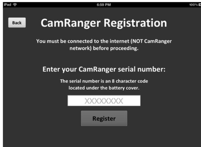
Enter the 8-character CamRanger serial number. The serial number is located both on the bottom of the back cover as well as above the battery underneath the back cover. Note: the serial number contains only letters and NO numbers.
